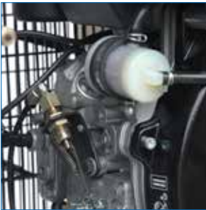
Device that reduces the engine speed for no load run
