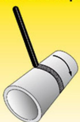
Pipe rotates with axis horizontal,
