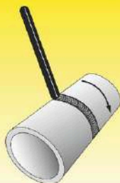
Pipe rotates with axis horizontal, welding downhand: PA/1G
