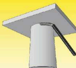
Pipe fixed with axis vertical, welding overhead: PD/4F
