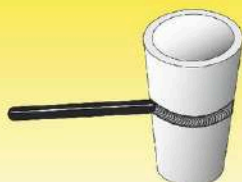
Pipe fixed with axis vertical, welding horizontal-vertical: PC/2G
