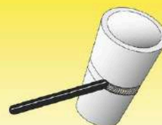
Pipe fixed with axis under 45° angle, welding upwards: H-LO45/6G
