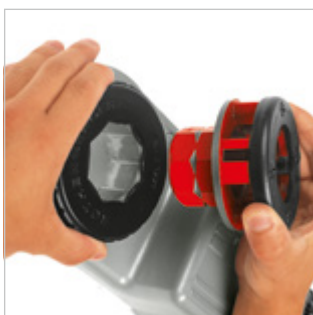
Easy insertion of the die heads
