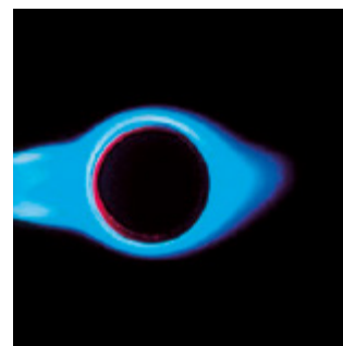
High flame temperature based on cyclone swirl
