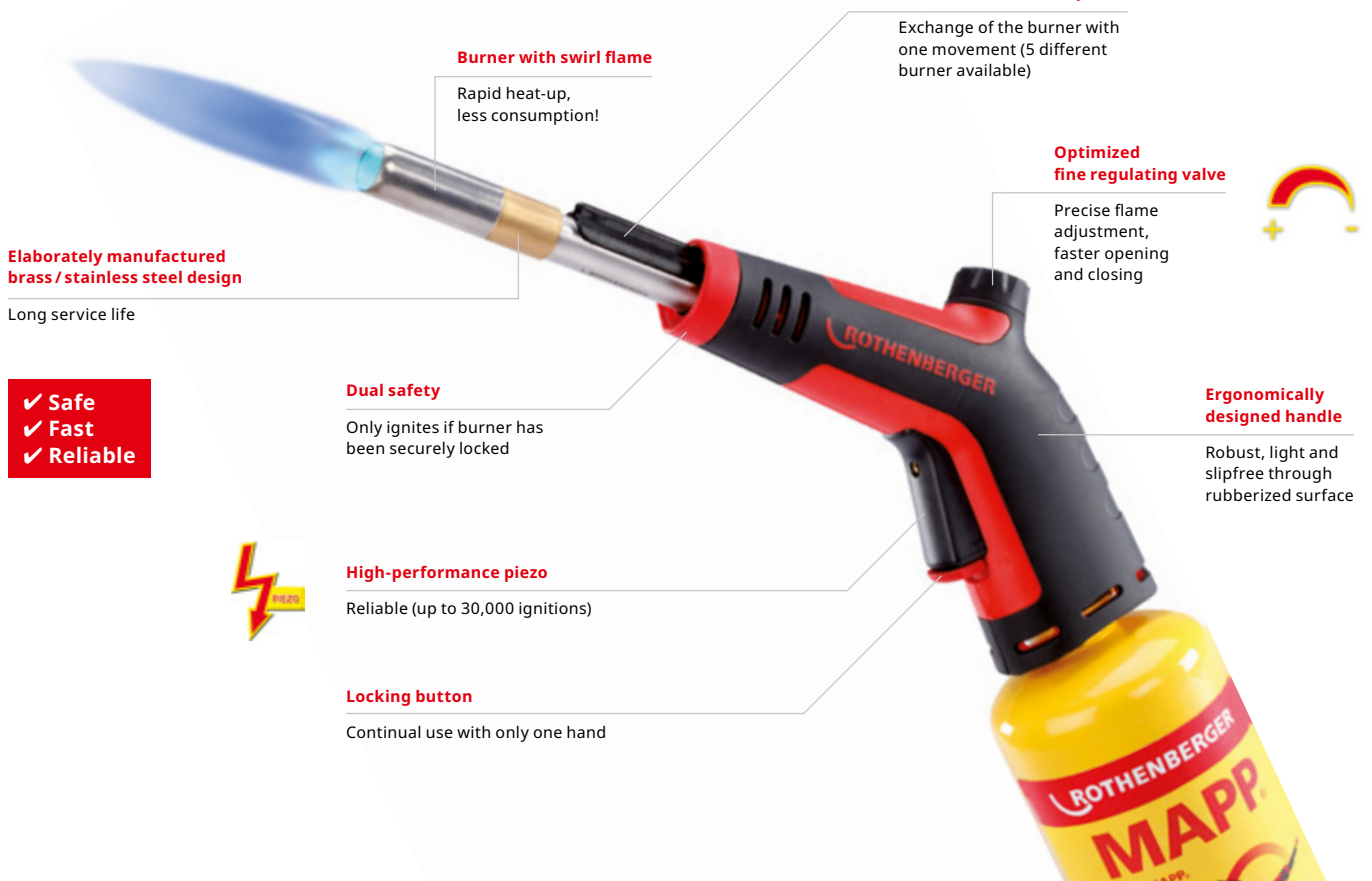
High flame temperature based on cyclone swirl
