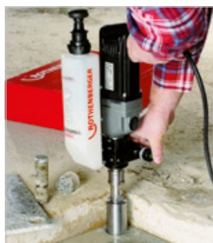
Drilling of the hardest materials
